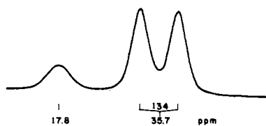
Fig. 4.— B^{11} n.m.r. spectrum of 1,7-B_{12}H_{10}[N(CH_3)_3]_2 in acetonitrile-dimethylformamide ( J in c.p.s.).
